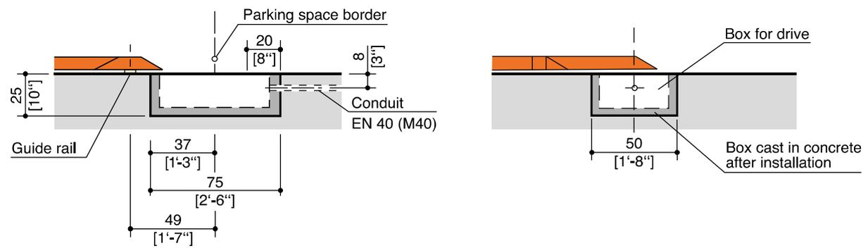
The drive housing does not provide complete protection against the ingress of running water. It must be ensured that no running water enters the area of the drive.
