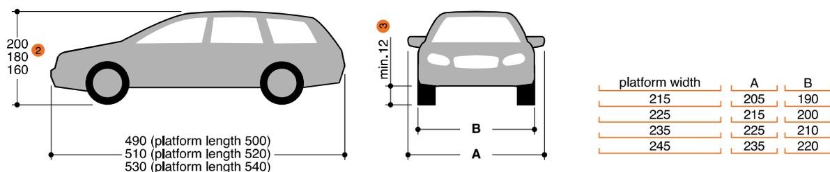
② Overall height (vehicle with roof racks, roof rails, aerials, etc. are not permitted to be higher than the specified height).
